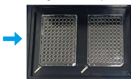
Exchanged to a 96 well plate adaptor (option)
