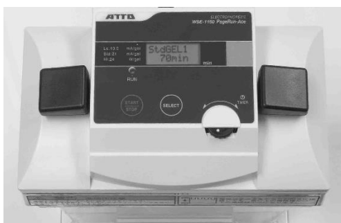
Integrated power supply module with safety cover
