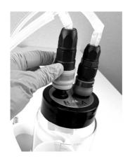
5. Separate the fitting part of suction nozzle A (handhold operator) and connect it to the silicone tube.
