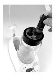
4. Connect the one-touch joint (Orange) to the B port on the reservoir cap.
