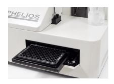
Push "PLATE" button to open and set the plate on the holder. Then push "PLATE" button again to close.
