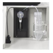
Prime injector line with appropriate reagents. Reagent volume for rinse and prime of injector line is only  $340\mu L$ .
