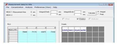
Measurement results of individual luminescent intensities are plotted at the interval of 20 msec
