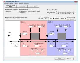
Select plate type (96/384 well plate) and set the measurement condition, such as injection volume, measurement time, delay time, filter and so on. Dual injectors (optional) are available, which allows to automatic analysis of dual reporter assay with two kinds of substrate reagents.
