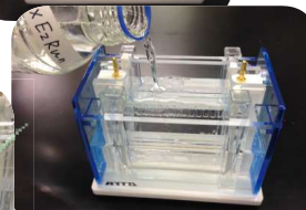
Pour electrode buffer to lower chamber. After setting upper chamber (gel), pour the buffer to it.
